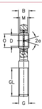
$\begin{array}{ll} A & = 24 \\ a \text{ (degrees)} & = 15 \\ B & = 8 \\ D & = 8 \\ D \text{ Dynamic drive (kN)} = 5.5 \end{array}$
